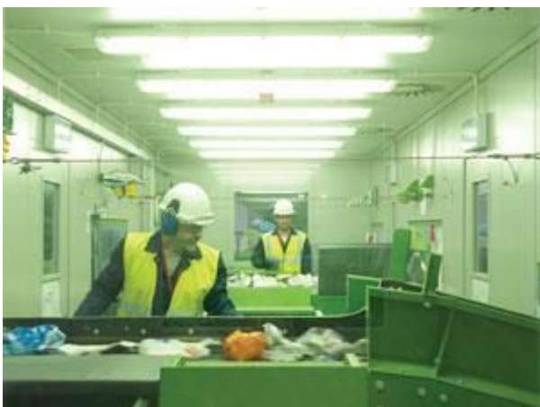
Trained human pickers remove any items that the sorting equipment won't be able to handle
