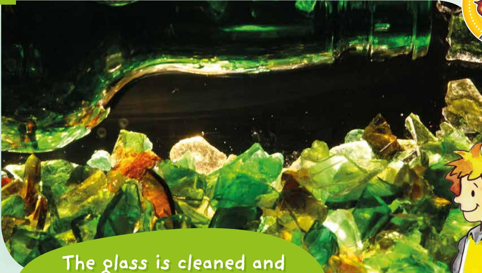
The glass is cleaned and crushed into what is called cullet and then ash, sand and limestone are added.
