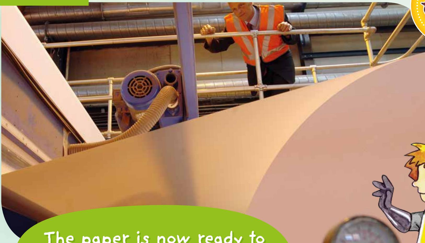
The paper is now ready to send through a big machine which squashes and flattens the pulp into giant sheets.
