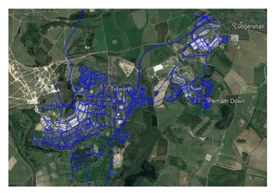
The Tidworth network consists of a single distribution system fed by the boreholes Chalkpit (CP) and Boreholes BH2 and BH3 via a service reservoir at Clarendon. The population and size of the network are such that it is classified as a single Water Resource Zone (WRZ) with major features shown in the map above.
