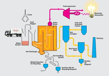
Waste not segregated for recycling or composting by residents is collected and transported to the Facility, where it is deposited into a bunker. A crane grabs the waste and places it into the feed hopper where it passes down onto the combustion grate. The action of the grate turns the waste to allow it to burn fully. The resulting ash then has metals extracted for recycling. The remaining ash is then sent for reprocessing and use as an aggregate substitute principally in road construction.
