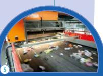
Near Infrared beams are used to detect plastic items and air jets blow them off the conveyer belt.
