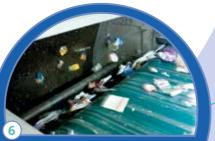
Eddy current produces a magnetic field which repels the aluminium from the rest of the material.
