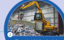
The material is then loaded into a bag splitter before the sorting process begins.
