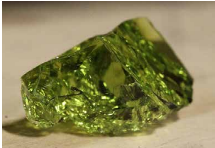
GeoMelt® has treated nuclear and hazardous waste since the 1990s and has produced over 26,000 metric tons of glass for storage.
